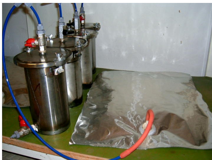
Fig. 2. Set of dry batch anaerobic reactors
